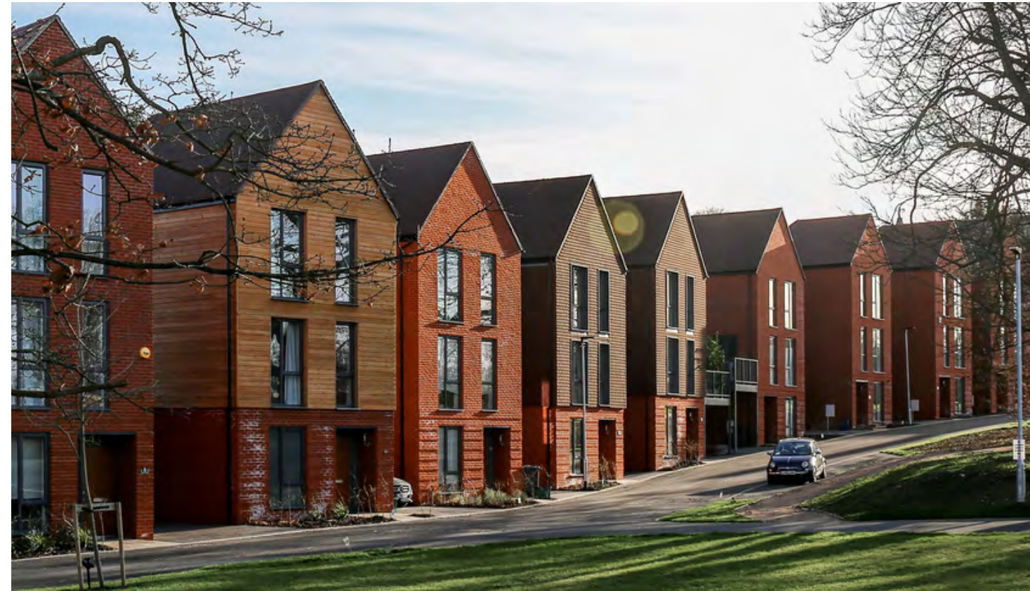
Figure 121. Gaps between houses to accommodate parking, creating a stronger relationship with the streets. Cane Hill, Croydon - HTA Design
